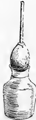
FIG. 6.—Osmosis with an egg over a bottle of water. The egg liquid and the water exchange places through the membrane of the egg. Water moves the faster and soon fills the shell to overflowing.
